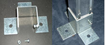
Step 4. Locate two of the ¼-20 x ¾" hex bolts (part J) and insert one into the slotted channel in the center of both sides of the Top Profile. Next locate one of the three remaining ¼-20 x ½" hex bolts and insert it on just one side of the Top Profile by placing the head into the slotted channel and sliding it onto the Top Profile (see photo below on left).
