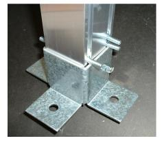
Step 5. Locate the remaining four ¼-20 x ¾" hex bolts (part J) and insert the head of each into each of the two channels on both slotted sides of the Bottom Profile (see photo above on right). Next locate the remaining two ¼-20 x ½" hex bolts and insert one in each channel of the Bottom Profile on the same side as you inserted the one in the top profile in step 4. Align this side of the Bottom Profile with the side of Top Profile on which you placed the single hex bolt
